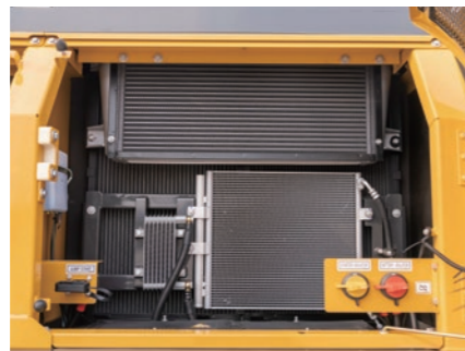
Series-parallel connection split type independent radiator.
