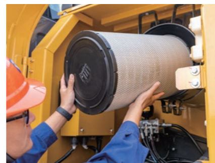
Air filter maintenance space is open, side door can be opened separately, easy maintenance.
