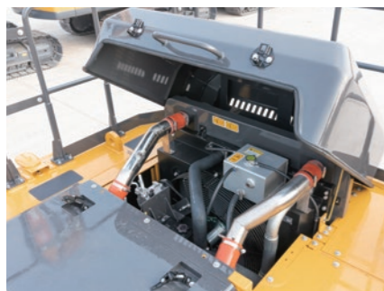
Large engine hood, opening Angle 75°, large engine room maintenance space.
